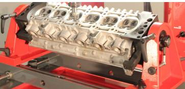
This feature allows a quick and easy mounting of the cylinder head while keeping a powerful clamping thanks to two jaws. It makes easier operations which require the access to different sides of the head.
