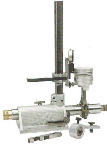
The illustration shows a connecting-rod being checked for bend. Control is done by checking the extremes of the piston pin, by simply moving the arbor.
