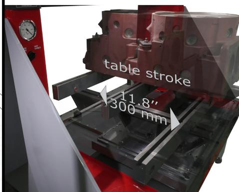
The support table is mounted on two guiding rails.
