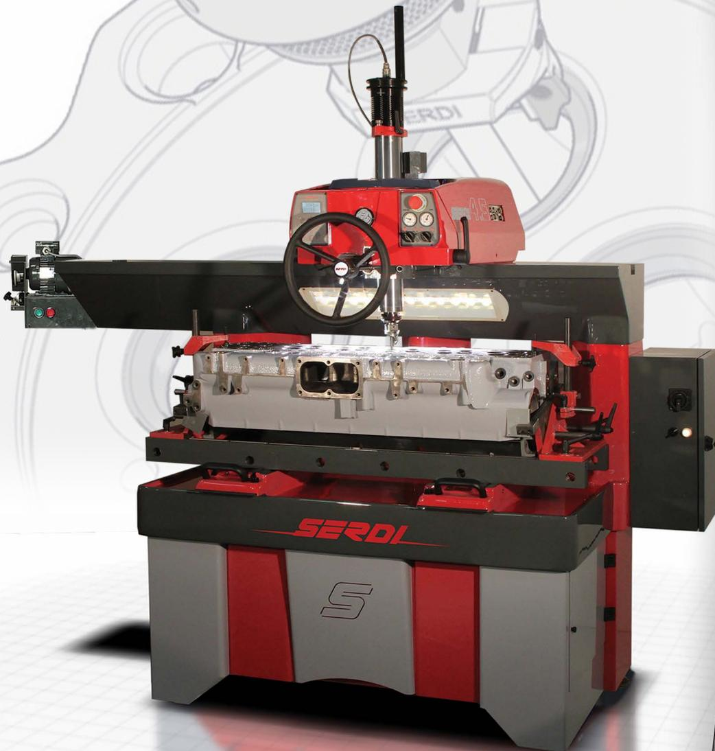
**Machining capacity from 16mm to 120mm / 0.6" to 4.72".**
