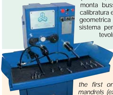
*This honing machine is a special version with two honing heads: on the first one you use expansion mandrels (ex. CM, GV etc...), while on the second one you use diamond tools for the geometric gauging and the roughness finishing of piece.*
