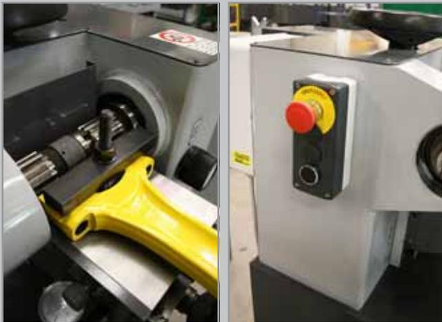
BL50 is designed for resurfacing the parting face of connecting rods and main bearing caps. The large capacity and robust construction make it ideally suited for both automotive and heavy duty diesel applications. The adjustable clamping mechanism allows the operator to surface caps on the original parting line even when the clamping surface is not square with this area. These features make it the ideal companion for rod and main bore resizing equipment.
