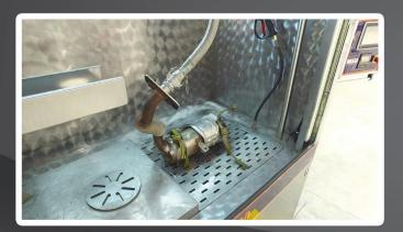
**DPF1800** is specially designed for Diesel Particul Filter cleaning. By the time, the particul filters for diesel engines get clogged and reduce the engines efficiency. In this case this filters need cleaning.
