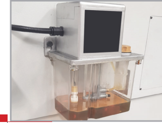
Otomatik yağlama sistemi Automatic lubrication system
